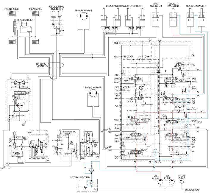
When the boom up and bucket in functions are operated simultaneously, the boom spools and bucket spool in the main control valve are moved to the functional position by the pilot oil pressure (XAb1, XAb2, XAk) from the remote control valve.
