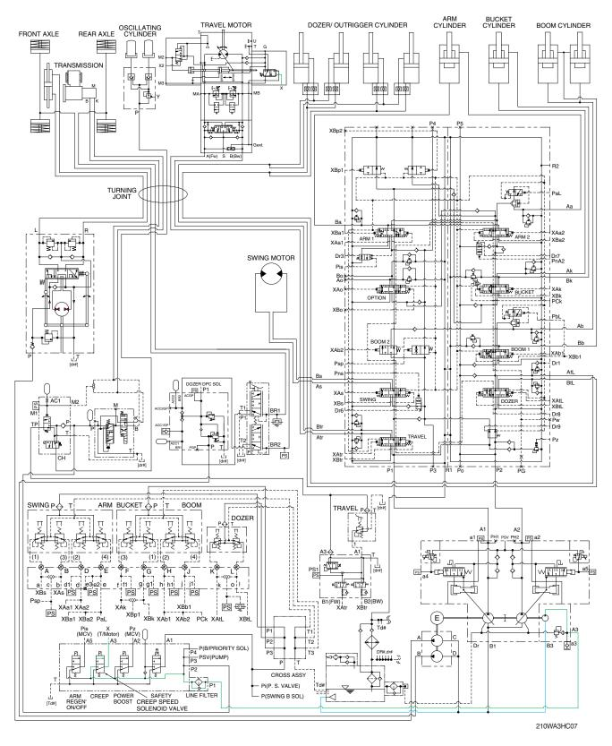
When the creep button on the dashboard of the steering column is pushed ON, the creep travel solenoid valve is actuated.
