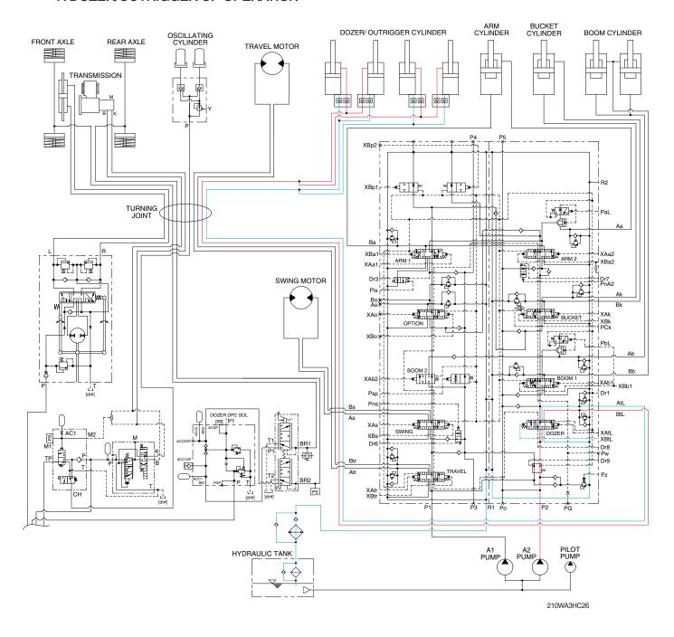
When the dozer control lever is pulled back, the dozer spool in the main control valve is moved to the dozer up position by the pilot oil pressure (XBtL) from the remote control valve.
