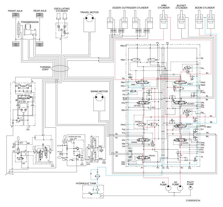
When the boom up and arm functions are operated simultaneously, the boom spools and arm spools in the main control valve are moved to the functional position by the pilot oil pressure (XAb1, XAb2, XBa1, XBa2, XAa1, XAa2) from the remote control valve.
