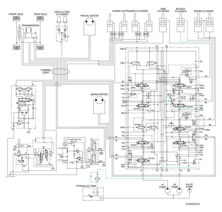
When the right control lever is pushed right, the bucket spool in the main control valve is moved to the bucket out position by the pilot oil pressure (XBk) from the remote control valve.
