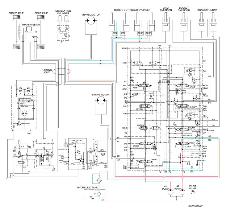
When the dozer control lever is pushed forward, the dozer spool in the main control valve is moved to the dozer down position by the pilot oil pressure (XAtL) from the remote control valve.
