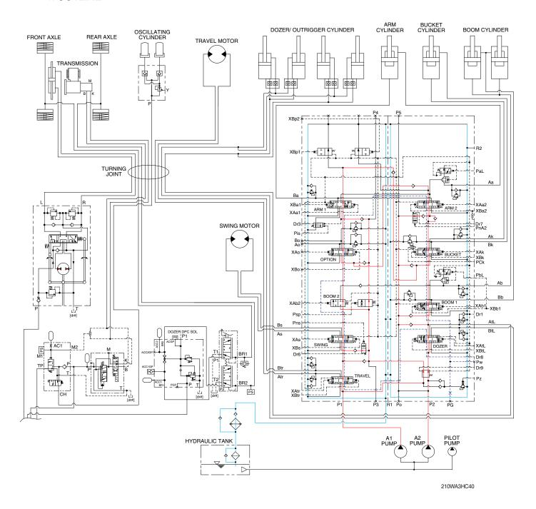
The oil from the A1 and A2 pump flows through the neutral oil passage, bypass oil passage and confluence oil passage in the main control valve. Then the oil goes to each actuator and operates them. Check valves and orifices are located on these oil passage in the main control valve. These control the oil from the main pumps so as to correspond to the operation of each actuator and smooth the combined operation.
