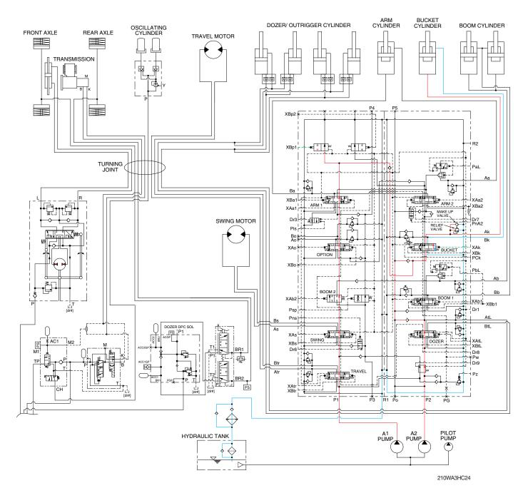
When the right control lever is pulled left, the bucket spool in the main control valve is moved to the roll in position by the pilot oil pressure (XAk) from the remote control valve.
