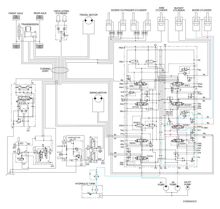
When the right control lever is pushed forward, the boom 1 spool in the main control valve is moved to the down position by the pilot oil pressure (XBb1) from the remote control valve.
