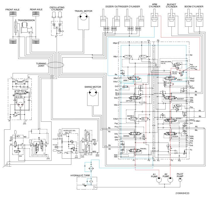
When the left control lever is pushed forward, the arm spools in the main control valve are moved to the arm out position by the pilot oil pressure (XAa1, XAa2) from the remote control valve.
