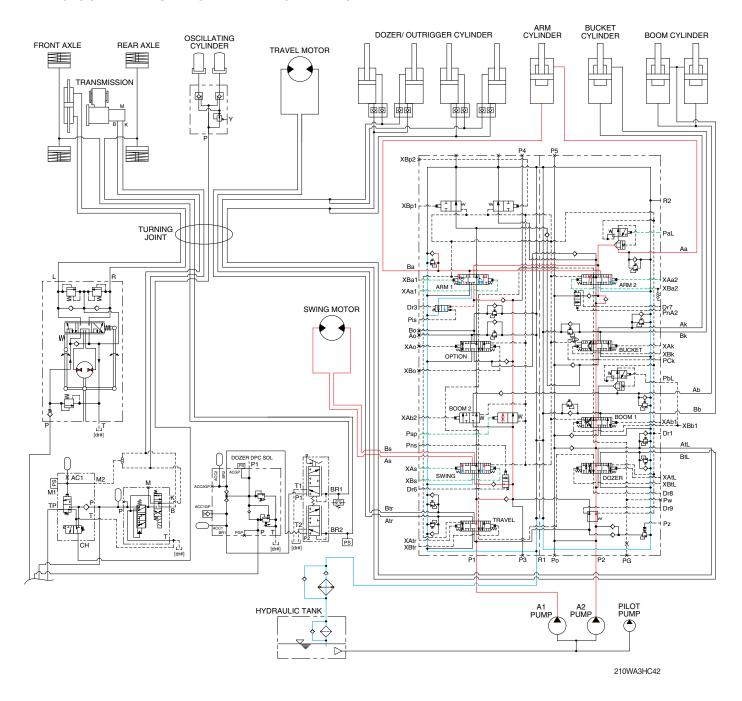
When the swing and arm functions are operated simultaneously, the swing spool and arm spools in the main control valve are moved to the functional position by the pilot oil pressure (XAs, XBs, XBa1, XBa2, XAa1, XAa2) from the remote control valve.
