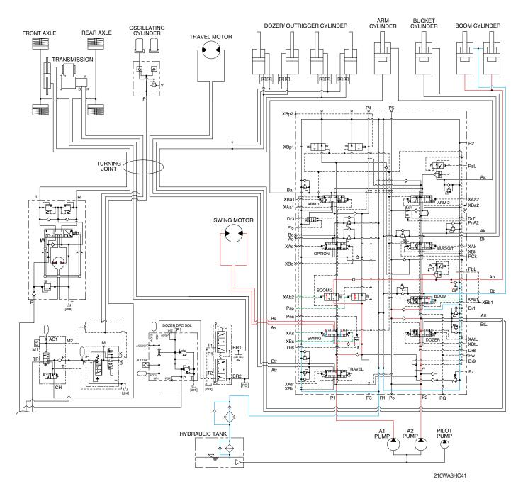
When the swing and boom up functions are operated simultaneously, the swing spool and boom spools in the main control valve are moved to the functional position by the pilot oil pressure (XAs, XBs, XAb1, XAb2) from the remote control valve.
