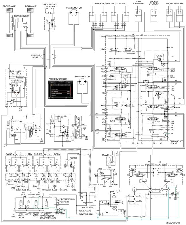
When the power boost switch on the left control lever is pushed ON, the power boost solenoid valve is actuated, the discharged oil from the pilot pump flows into **Pz** port of the main relief valve in main control valve; then the setting pressure of the main relief valve is raises from 350 kgf/cm² to 380 kgf/cm² for increasing the digging power. And even when press continuously, it is canceled after 8 seconds.
