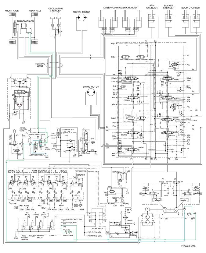
When LH multifunction switch was placed in high or low speed position, the pressure oil from pilot pump flows to travel speed solenoid valve through travel control valve, thus the transmission is changed into high (B) or low (K) speed condition.
