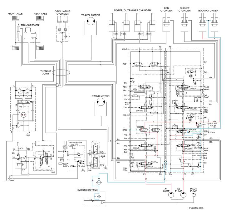
When the right control lever is pulled back, the boom spools in the main control valve are moved to the up position by the pilot oil pressure (XAb1, XAb2) from the remote control valve.
