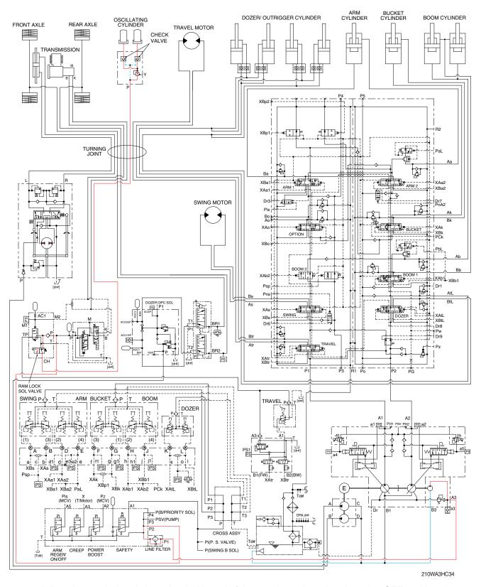
When the ram lock switch on the dashboard of the steering column is selected to OFF position, the ram lock solenoid is changed over.
