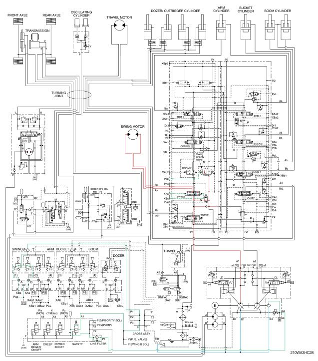
When the left control lever is pushed left or right, the swing spool in the main control valve is moved to the left or right swing position by the pilot oil pressure from the remote control valve. Also the swing operation preference function is operated by the pilot pressure **Psp** (refer to page 3-17).
