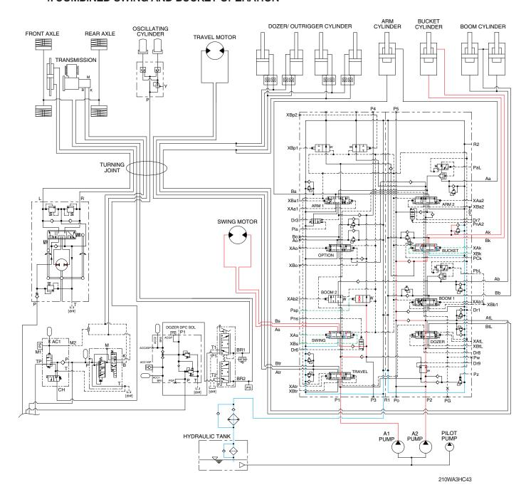
When the swing and bucket functions are operated simultaneously, the swing spool and bucket spool in the main control valve are moved to the functional position by the pilot oil pressure (XAs, XBs, XAk, XBk) from the remote control valve.
