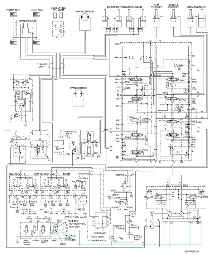
When the knob of the safety solenoid valve is in the release position, oil flows into the remote control valve through the line filter, safety solenoid valve and cross assy.
