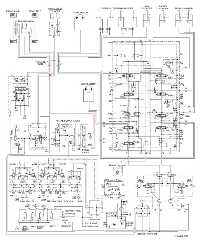
When the brake pedal (valve) is pushed, the discharged oil from the power train pump (B) flows into the front and rear axle brake disc through the solenoid valve of brake supply valve.
