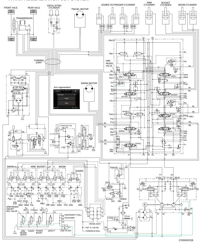
When the arm regeneration is selected to disable on the cluster, the arm regeneration solenoid valve is activated. The pilot oil from pilot pump flows into **Pis** port in main control valve through solenoid valve and the arm regeneration spool is shifted to left.
