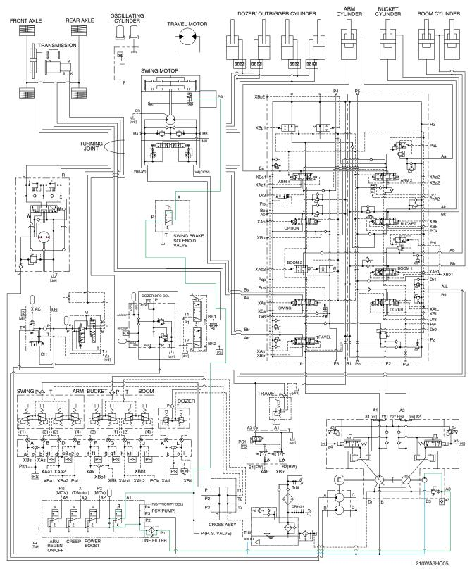
When any one of the swing, arm in or boom up lever is tilted, the swing brake solenoid valve is shifted to the down ward by the MCU that senses the pilot pressure of the swing control lever.
