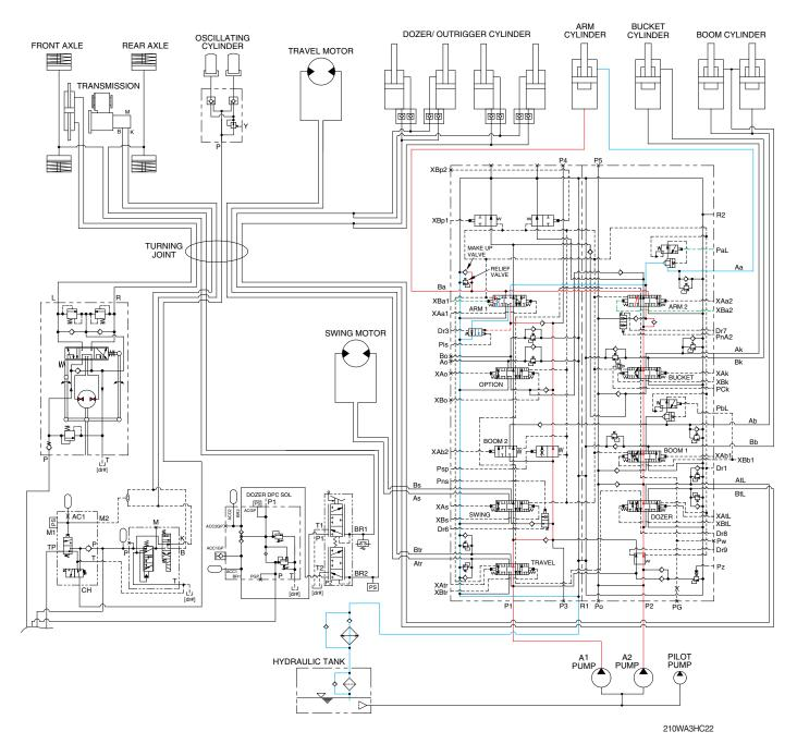
When the left control lever is pulled back, the arm spools in the main control valve are moved to the arm in position by the pilot oil pressure (XBa1, XBa2) from the remote control valve.
